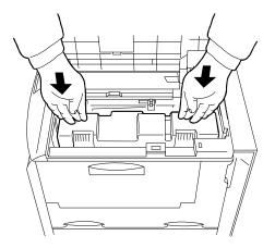
**10.** After the toner container is installed, slide the two toner container release levers to the left position (fixed) as shown in the figure.
